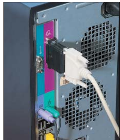
ESP LA-5/25 installed on the parallel port of a PC, protecting the printer connection
