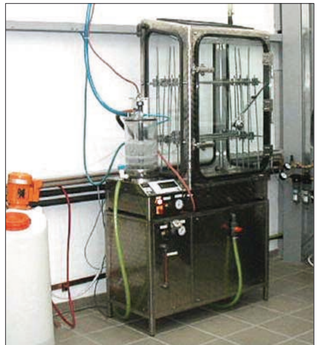
Environmental ageing chamber for ammonia atmosphere ageing
